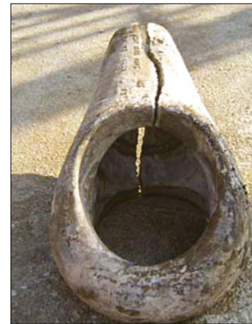
Shaker: mooring socket failures add to shackle woes Photo: MMS
