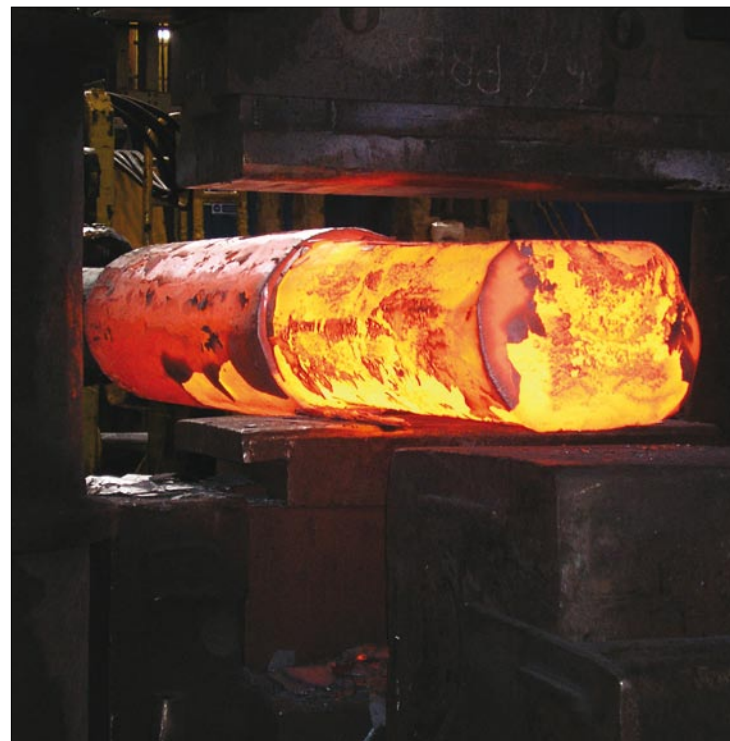
Back to basics: new research project aims to gain better understanding of the integrity of mooring components formed by the hot deformation of steel that is the forging process Photos: FIRST SUBSEA
